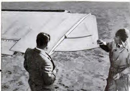
Extended by the pilot before landing, the wing tips steady a plane
